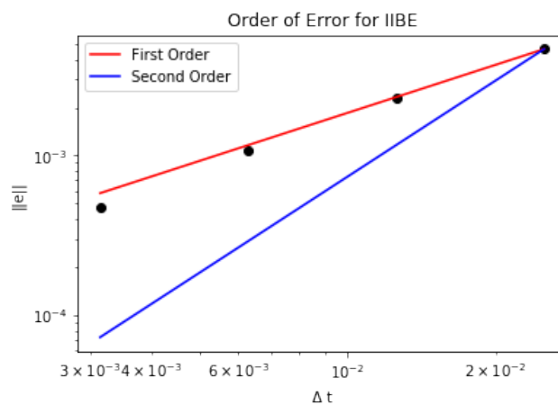
Figure 10: In this figure we show the convergence of error for the IIBE method with respect to time is order 1.
